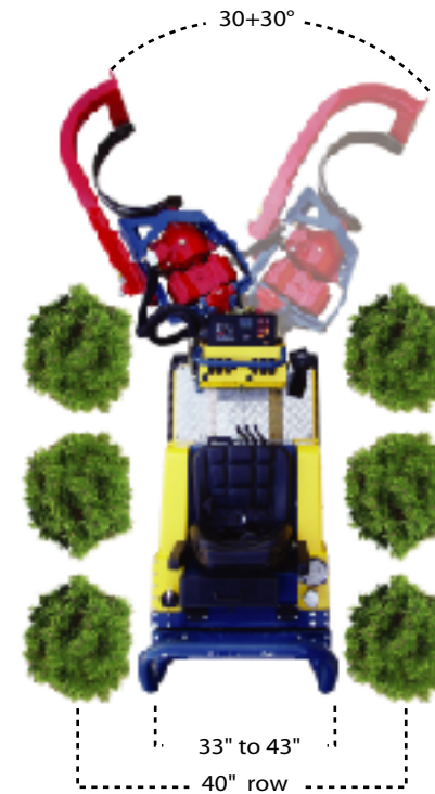
Rotating Digging Head
